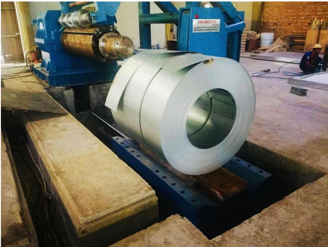
TOKO Slitting Line (from Africa Customer's Factory)
