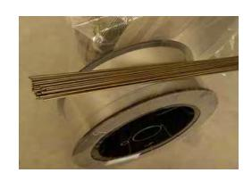
Euro Tig Monel 7 is used for TIG and MIG welding of nickel copper alloys(ASTM B127,B163,B164 and B165 UNS Number No4400). This filler metal can be used for MIG overlay on steel after a first layer with nickel 208(Filler Metal 61). Dissimiliar welding applications include joining nickel copper alloys to Nickel 200 and copper nickel alloys.
